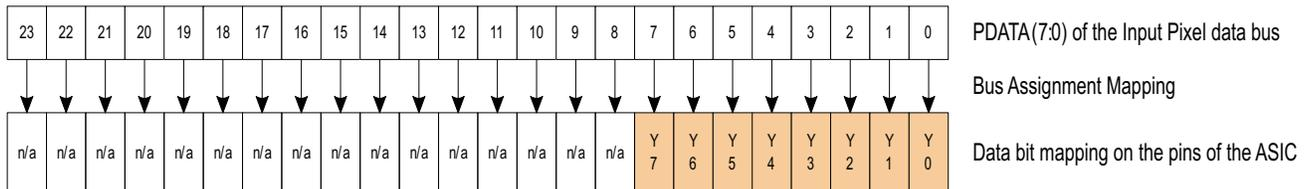
**Figure 14. PDATA Bus – BT.656 I/F Mode Bit Mapping**
