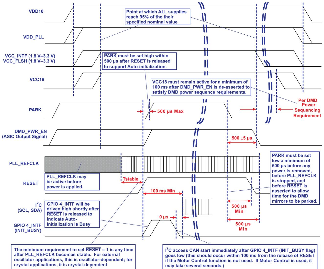
Figure 19. Power-Up/Down Timing
