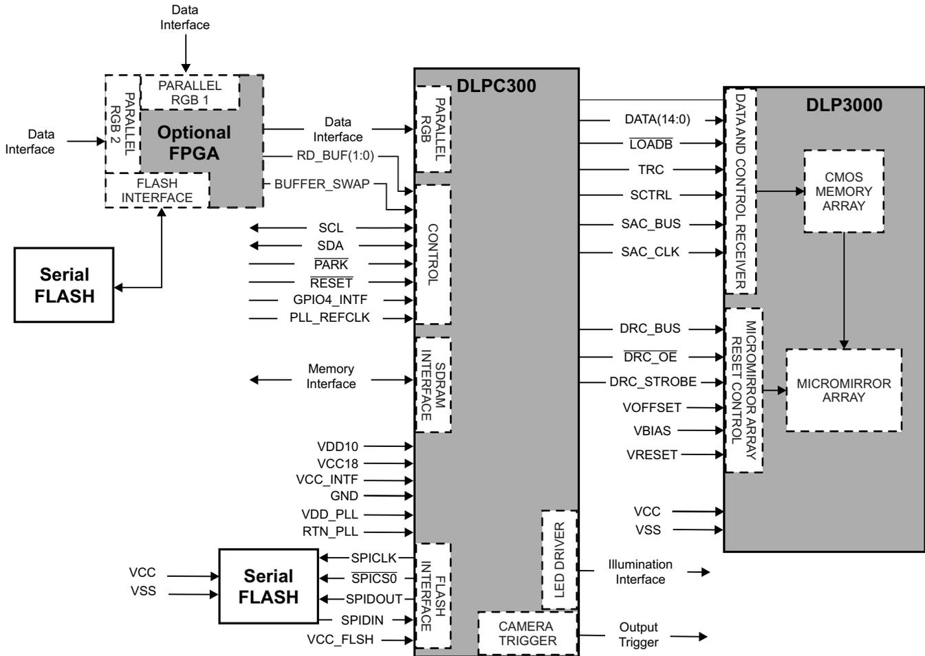
Figure 6. DLP3000 Chipset With Optional FPGA
