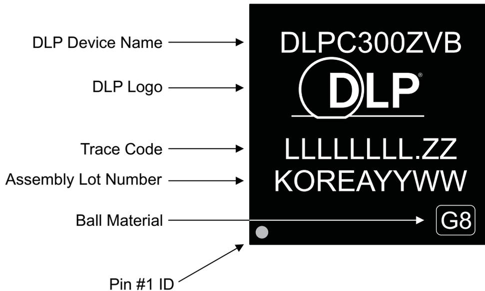
Figure 9. Device Marking
