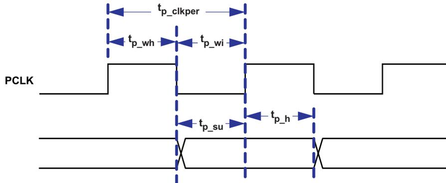
Figure 13. Parallel and BT.656 I/F General Timing
