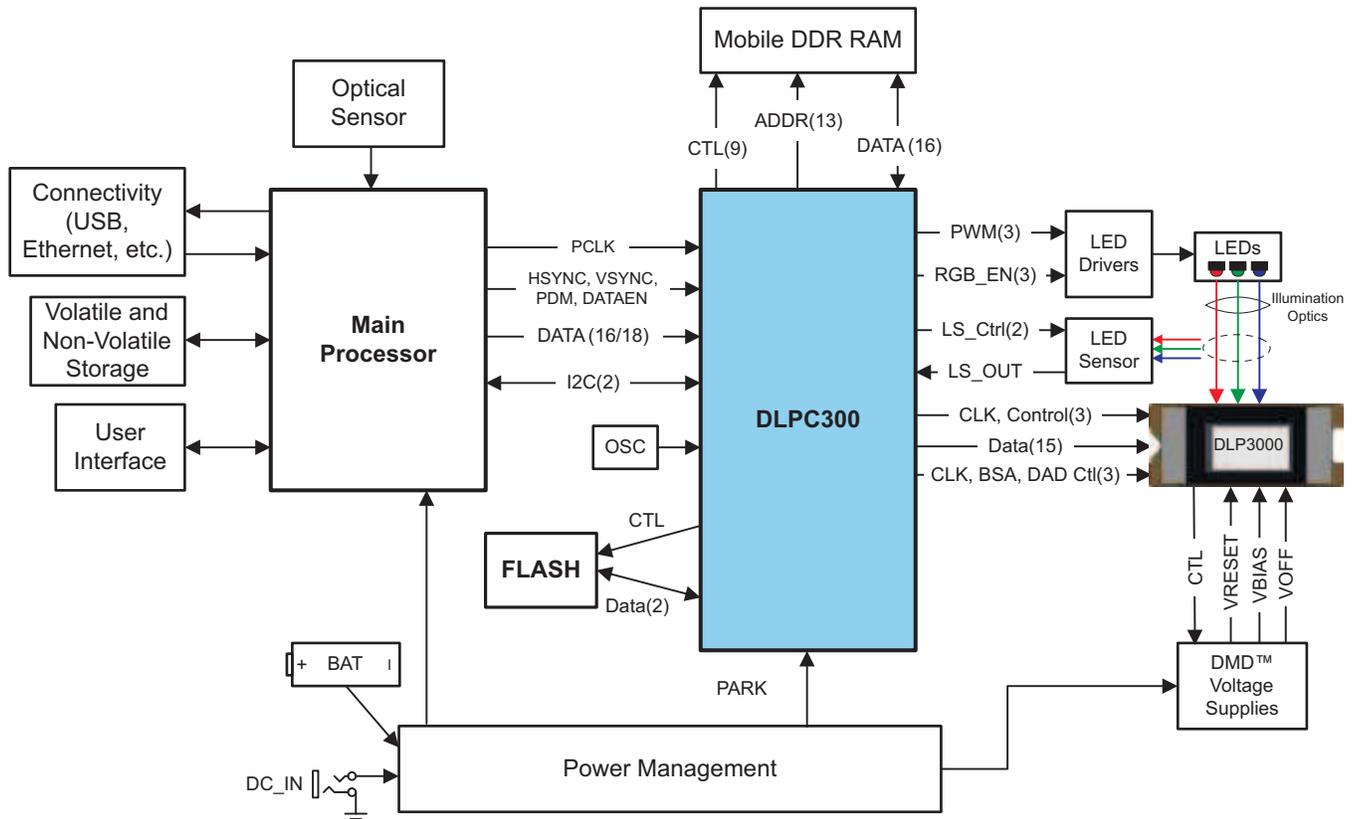
Figure 7. Typical Embedded System Block Diagram
